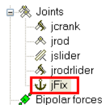
Figure 3.176. Icon of a fixation joint in the element tree
