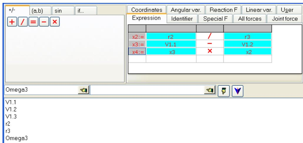
Figure 4.95. Expressions for computation of angular velocity of the planet gear
